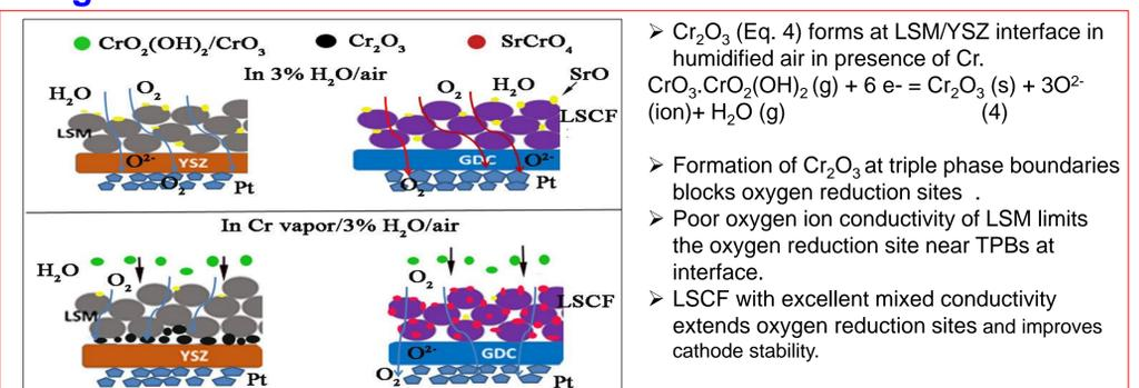
Figure 7. Schematic of the degradation mechanisms of LSM and LSCF cathodes in air containing H<sub>2</sub>O and chromium vapor.
