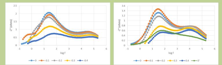
Fig. 7: Bode plots of the cell at constant cell voltage after 120 s at the same cell voltage.
