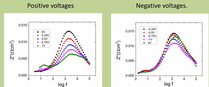
Fig. 3: Bode plots of the LSCF/YSZ/LSCF cell with respect to applied cell voltage after 120 s conditioning at each voltage. The Z'' data is corrected for the two electrodes.
