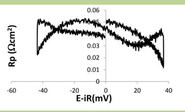
Fig. 1: Cyclic voltammety at 1000 mV/s illustrating nearly ohmic behavior of a symmetrical cell with LSCF electrodes at 800°C in air.
