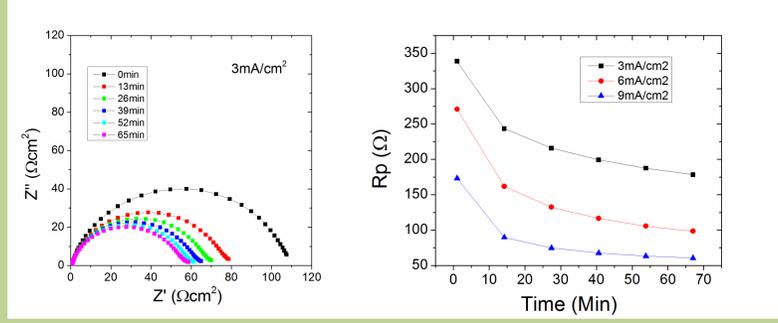
Fig. 5: Under small current (3, 6, 9 mA/cm<sup>2</sup>), the polarization resistance of LSM electrode was reduced to 53%, 41% and 36% within 1 hour. The polarization resistance of the LSCF CTR electrode is negligible on this scale.
