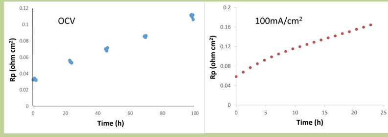
Fig. 4: Over 100 hour in air at 800°C under OCV, the polarization resistance nearly triples. Passing current leads to accelerated degradation.
