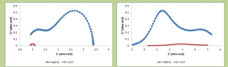
Fig. 6: Nyquist and Bode plots of the cell compared with the LSCF CTR electrode impedance from symmetrical cell studies.
