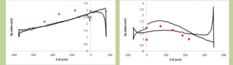
Fig. 8: Comparison of polarization resistances of the LSM/YSZ composite electrode as a function of applied DC voltage. Solid black lines from cyclic voltammograms, red circles from impedance measurements.
