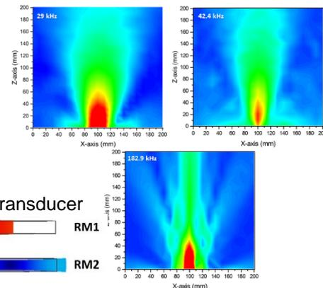
Radial modes of a Bessel-like transducer
