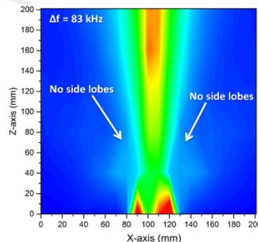
83 kHz difference frequency beam profile in H<sub>2</sub>O
