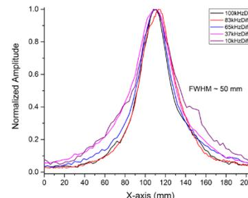
Scans of beam widths at 110 mm from transmitter in H<sub>2</sub>O
