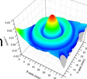
Examples for low-frequency beam profiles in H<sub>2</sub>O for a Bessel-like source
