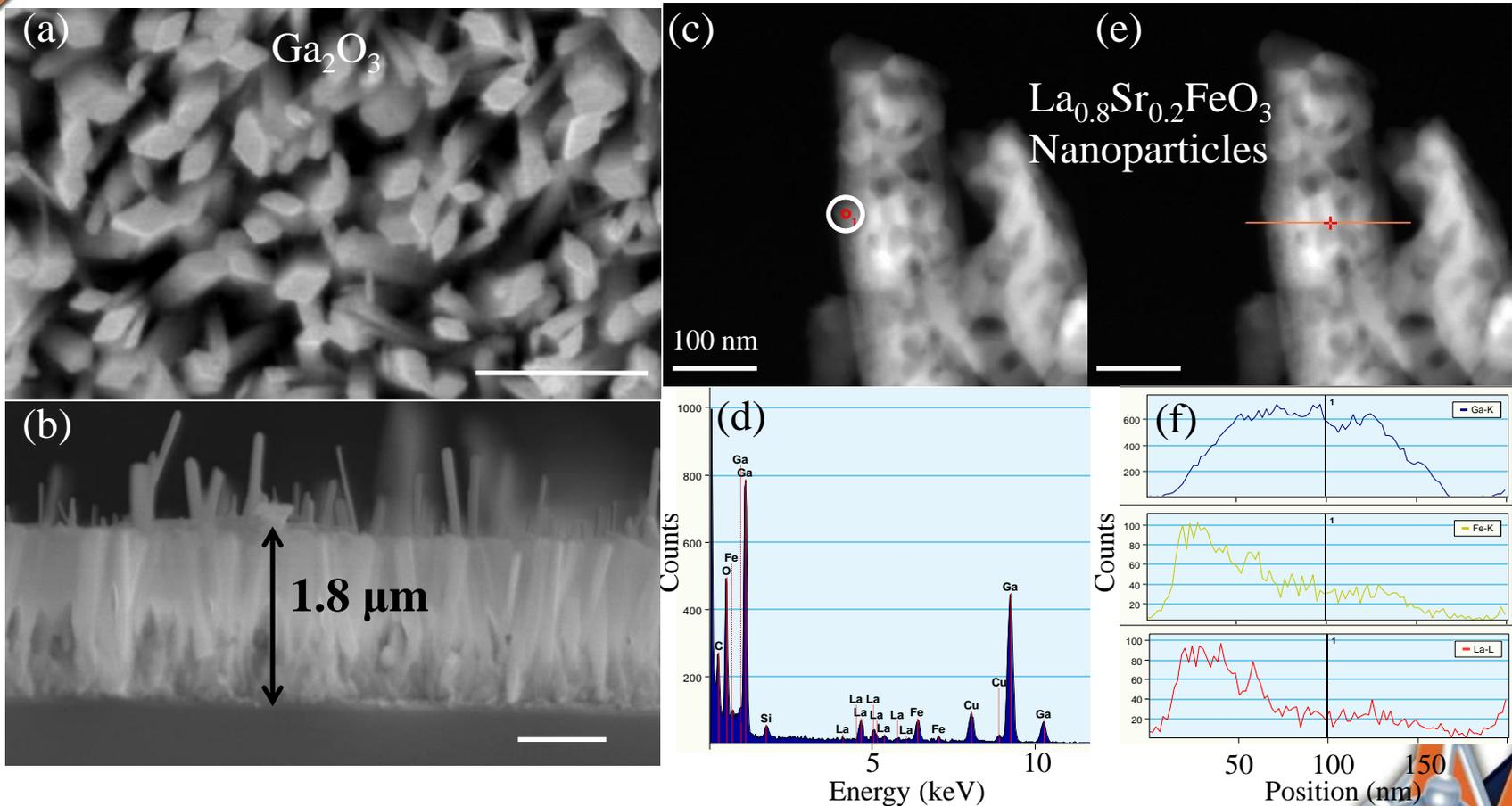
Figure 1: Top view (a) and (b) cross-sectional view SEM image of  $\text{Ga}_2\text{O}_3$  nanorods array. (c) (e) STEM images of a LSFO decorated  $\beta\text{-Ga}_2\text{O}_3$  nanorod showing its porous structure; the corresponding EDX spectrum of (d) point scanning, (f) line scanning revealing the existence and distribution of LSFO composition on  $\beta\text{-Ga}_2\text{O}_3$ .
