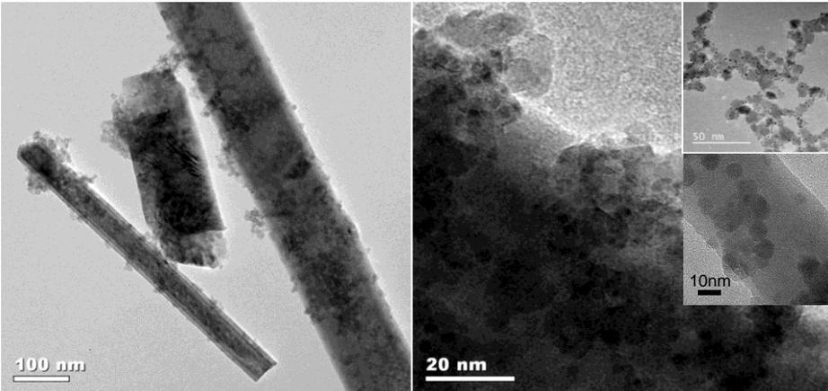
Hybrid nanoparticles on nanowires
