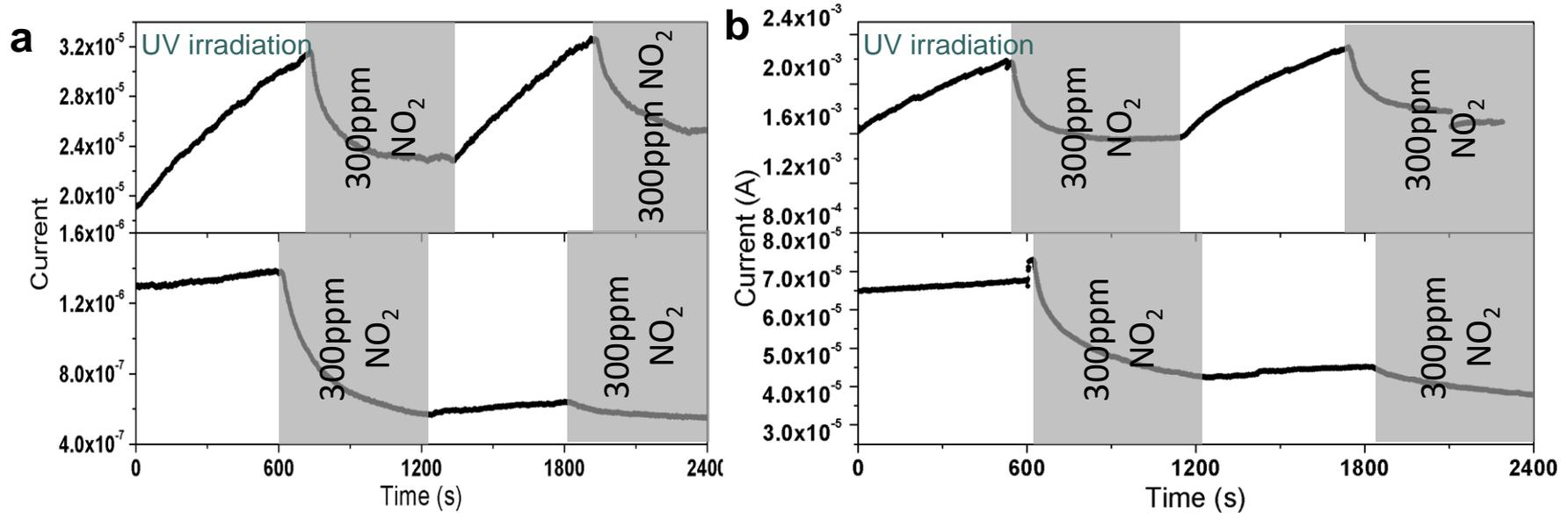
300ppm NO<sub>2</sub> and N<sub>2</sub> balance, room temperature, 1500sccm
