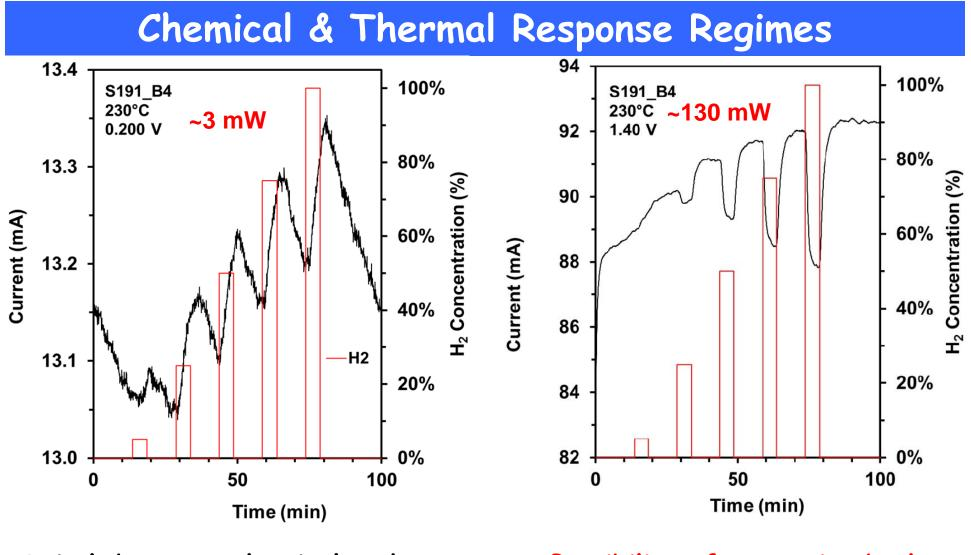
Switch between chemical and thermal response regimes by controlling operational power level Possibility of measuring both composition & flow characteristics using same sensor
