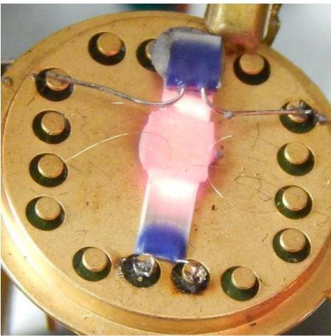
Sensor mounted 16 pin transistor outline header with microheater & RTD for temperature control & readout (Temperatures ≤800 °C)
