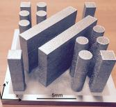
Bars ~3.5" tall + 3.5"x4" rectangular block Machining of conventional and small dog bone specimens for tensile and creep testing Characterization of the mechanical properties in different directions and annealing conditions
