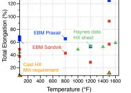
EBM HX alloys exhibit excellent ductility in the as fabricated condition at all temperatures
