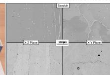
· Elongated grains along the build direction with both powders · Presence of small voids plus few larger voids due to entrapped
