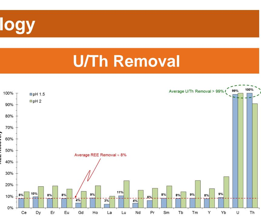
Selective removal of uranium (U) and thorium (Th) from rare earth elements (REEs) in a fly ash digest liquor. At pH 1.5, REEs separation is minimal while U/Th separation is maximized.
