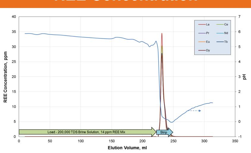
Tusaar media eluent containing concentrated, well separated REEs during extraction of metals from ligand modified activated carbon surface.
