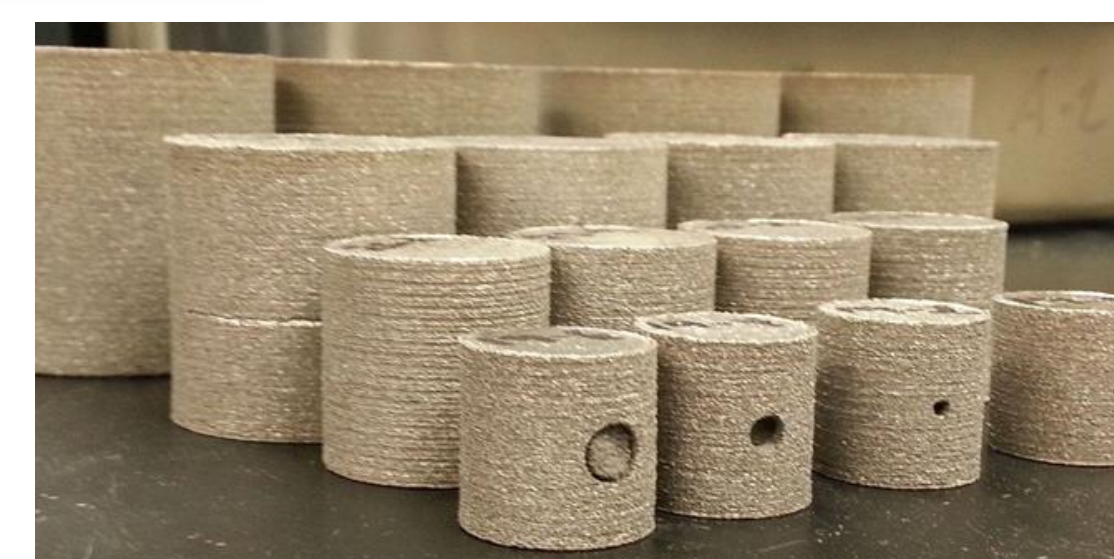
Test parts fabricated from different machine models a) A2X, b) A3, c) S12
