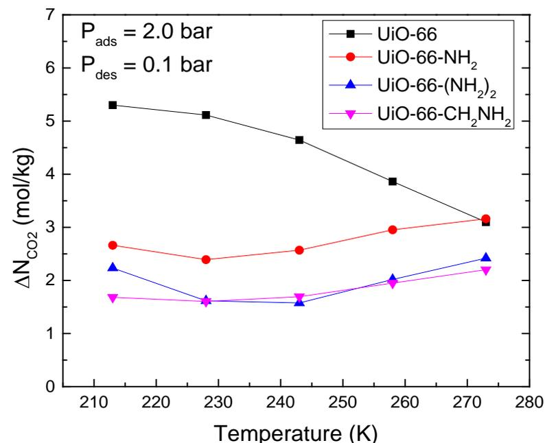
UiO-66 can achieve impressive swing capacities at sub-ambient conditions—but higher pore volumes needed for 10+ mol/kg
