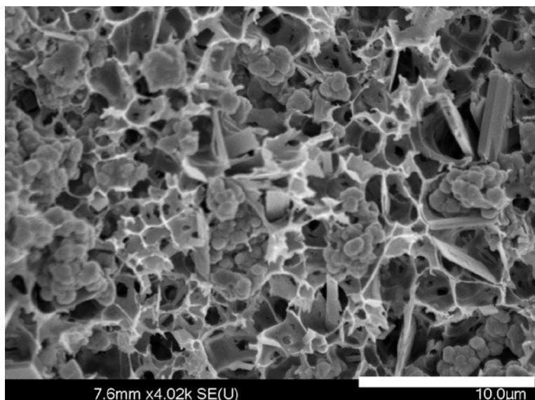
Water stable MOFs retain crystallinity and porosity after fiber sorbent spinning
