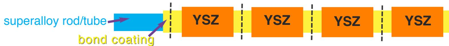
~4 specimens from each rod/tube: 100h cycles
