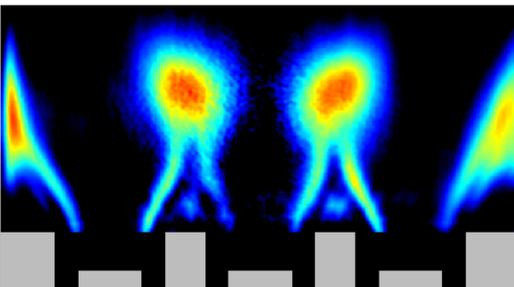
Slides through the flame shows center flame lift-off and significant flame-wall interaction at  $\phi = 0.48$
