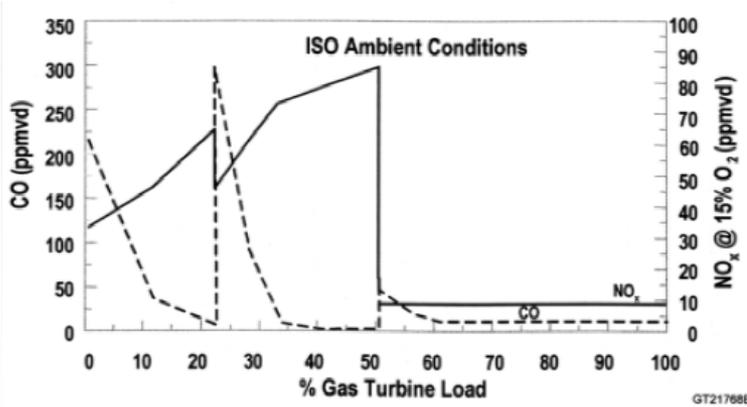
Figure 9. MS7001EA/MS9001E emissions - natural gas fuel
