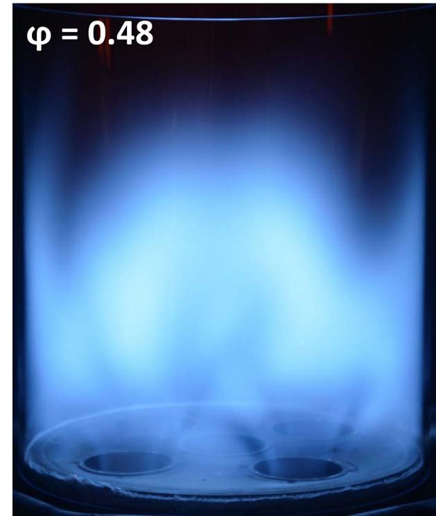
Photographs of multi-nozzle flame at  $U = 25$  m/s,  $T_{in} = 200^\circ\text{C}$
