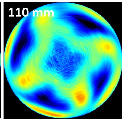
Flame-flame interaction dominates at  $\phi = 0.6$  and center flame, now attached, shows significant non-axisymmetry
