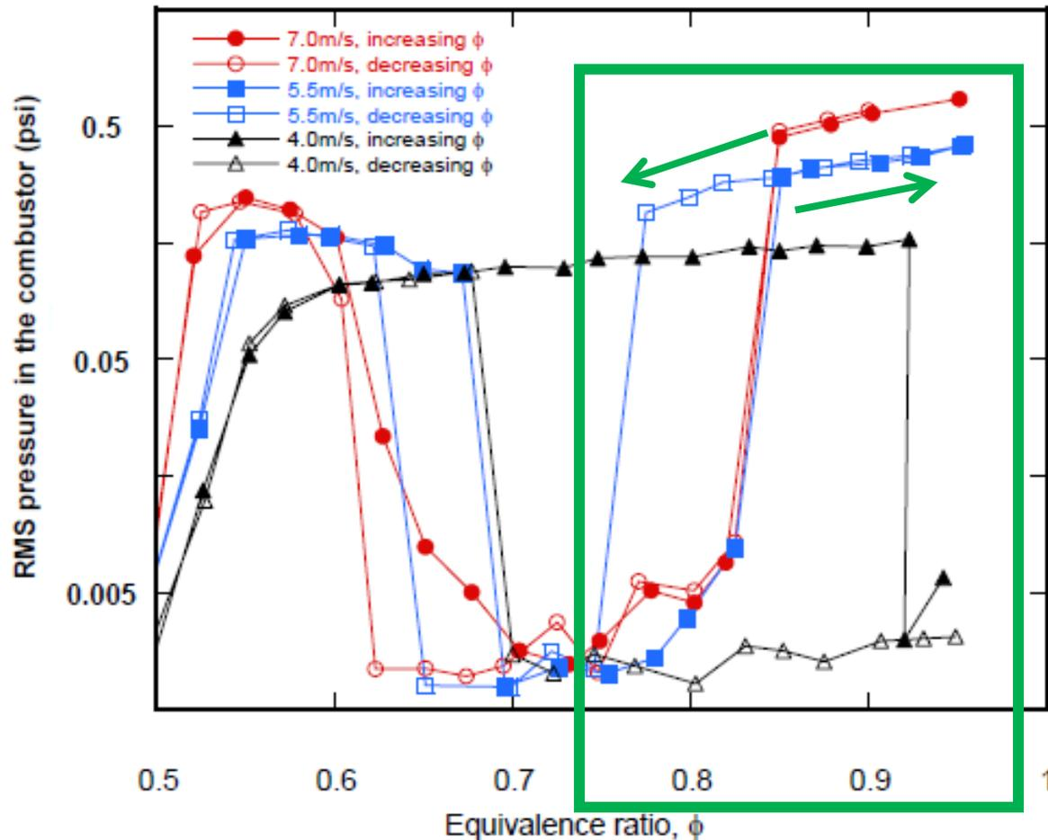
Instabilities may arise as a result of changes in flame shape and flame anchoring that occur with variation in equivalence ratio
