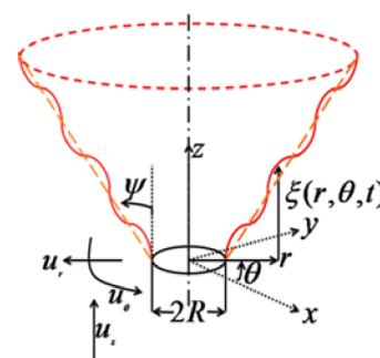
$$\frac{\partial \xi}{\partial t} + u_r \frac{\partial \xi}{\partial r} + \frac{u_\theta}{r} \frac{\partial \xi}{\partial \theta} + s_L \left[ \left( \frac{\partial \xi}{\partial r} \right)^2 + \frac{1}{r^2} \left( \frac{\partial \xi}{\partial \theta} \right)^2 + 1 \right]^{1/2} = u_z$$
