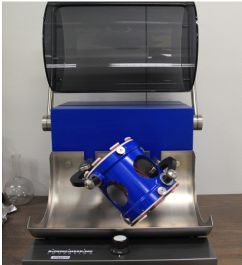
3-D inversion kinematics mixer (Inversina 2L)
