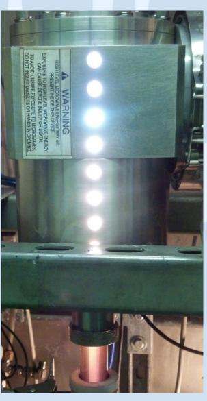
• Solid hydrocarbon particles are rapidly and selectively heated to pyrolytic temperatures (over 1000°C within 100 milliseconds). • Pyrolysis products (liquids) are immediately hydrogenated insitu with ionized and activated hydrogen-rich transport gases.
