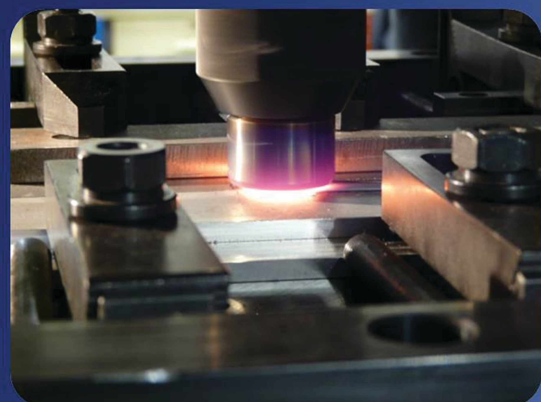
Friction stir welding of 1/4" thick dispersion strengthened Sandvik APMT plate
