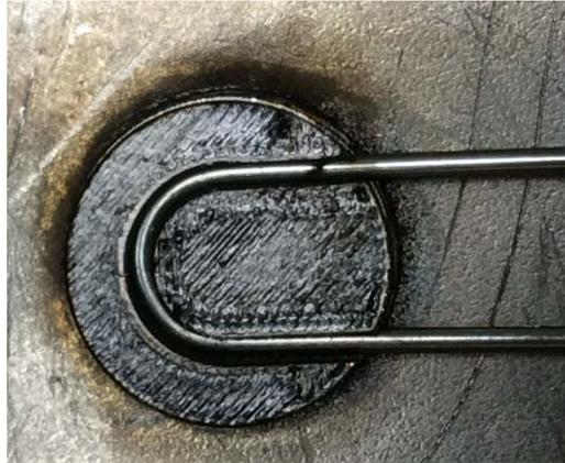
A curved sensor to be embedded in the printing process.
