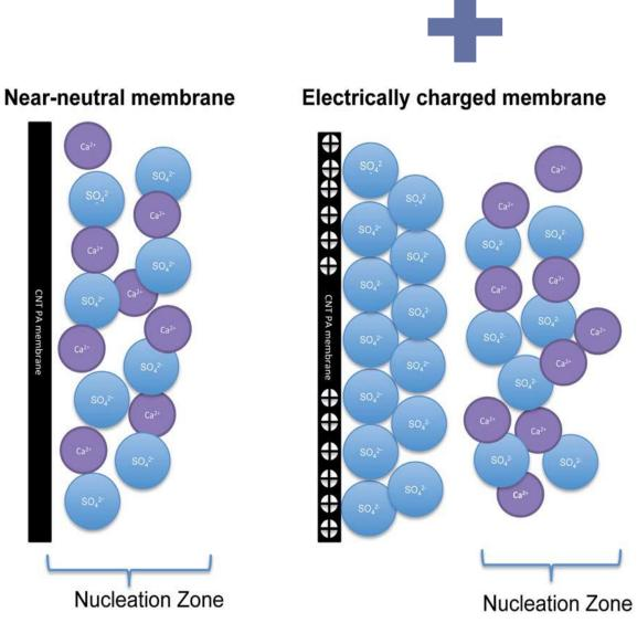
**Charged membrane** surface alters the mechanism by which scale is formed Nucleation zone is "pushed" away from the surface. Crystal formation occurs primarily in the diffuse layer
