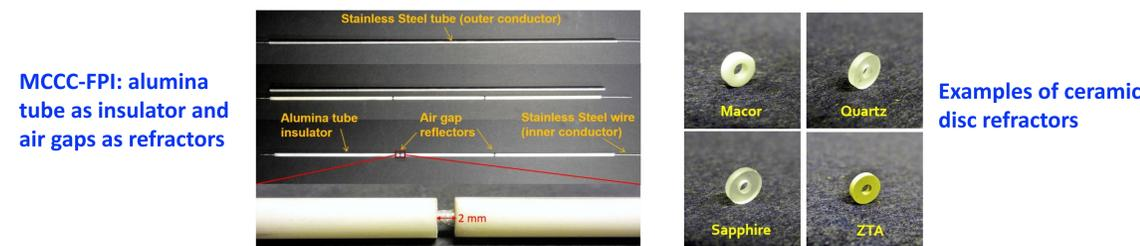
(Note: all MCCC-FPI sensors reported here used stainless steel tube and wire as outer and inner conductors, respectively.)
