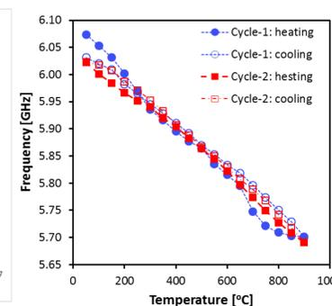
Correlation between temperature and wavelength shift for the MCCC-FPI with alumina insulator and air gap refractors
