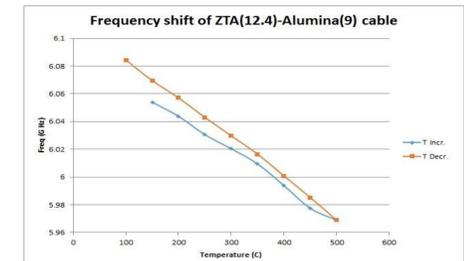
Correlation between temperature and wavelength shift for the MCCC-FPI with alumina insulator and Macor disc refractors
