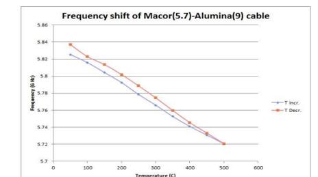
**Results/Observations:** For all MCCC-FPI sensors, the wavelength shift exhibited generally linear dependence on temperature up to 900°C (current test limit); consistency of temperature measurement improved by thermal cycles.
