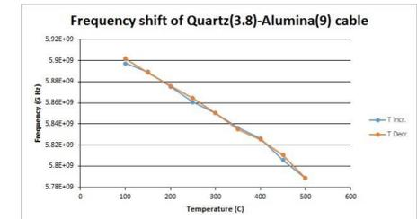
Correlation between temperature and wavelength shift for the MCCC-FPI with alumina insulator and ZTA disc refractors
