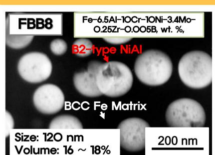
TEM dark field image of FBB8 along [100] zone axis using <100> superlattice
