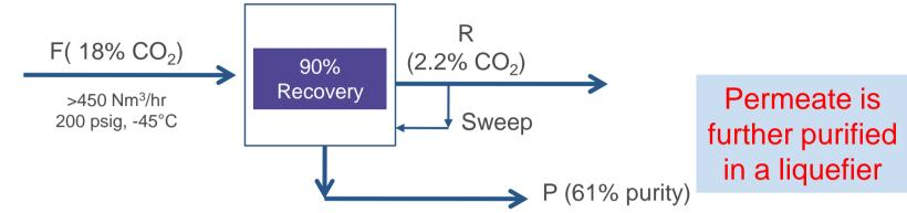
2 Stage Configuration in Series – Completed bench scale test (0.1 MWe) at different feed composition to validate the concept
