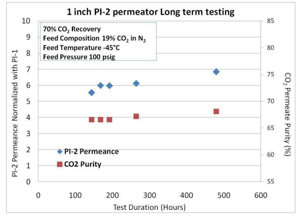
Performance is stable after >500 hours long term testing at cold temperature
