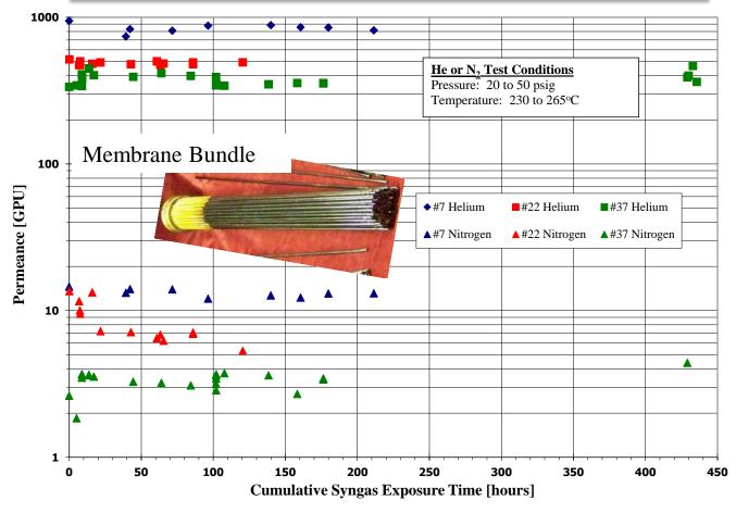
Performance stability of multiple tube CMS membrane bundles during  $H_2$  recovery from NCCC slip stream testing. He and  $N_2$  Permeances measured periodically during >400 hr test.
