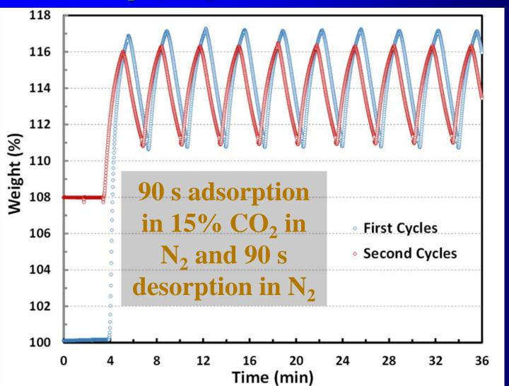
sample exposed to 2.5 hr of 42 ppm of SO, in  $N_2$ between sets of cycling tests – no regeneration
