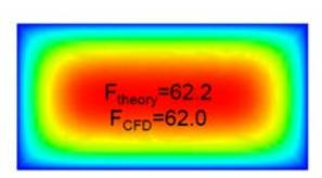
Best Shape Estimates from Rapid 1D Model Based on Parameters from 3-D CFD Models
