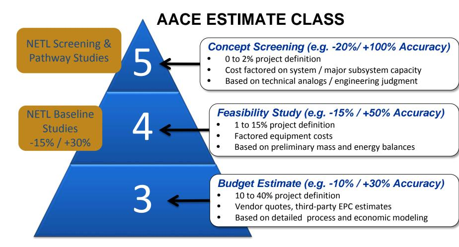
Process flow diagrams (PFDs) and piping and instrument diagrams (P&IDs) are the primary documents that define project scope. Association for the Advancement of Cost Engineering International (AACE) Recommended Practice No. 18R-97 describes the AACE cost estimate classification system.
