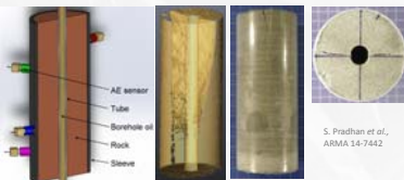
We are analyzing small rock samples acquired on a Missouri field trip. One strong sample from a road cut and one friable, weak sample from the Summit Proppant quarry were Scratch tested, porosity and permeability, thin section, bulk X-ray diffraction (XRD), and \mu CT imaging. Photos - SINTEF
