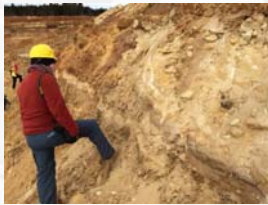
We are analyzing small rock samples acquired on a Missouri field trip. One strong sample from a road cut and one friable, weak sample from the Summit Proppant quarry were Scratch tested, porosity and permeability, thin section, bulk X-ray diffraction (XRD), and \mu CT imaging. Photos - SINTEF
