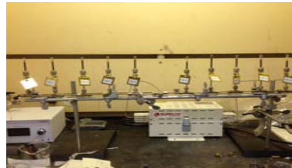
Sample tubes collected in the field, are dried for at least 2 hours with ultra high purity helium.
