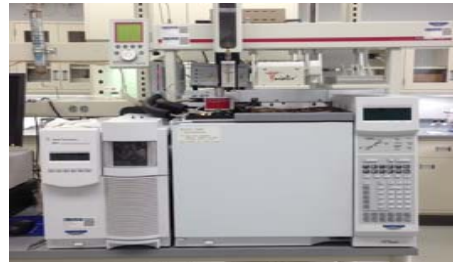
Agilent® 6890N gas chromatograph (GC) Gerstel® cryogenic focusing unit with autosampler Agilent® 5975 mass selective detector (MSD)
