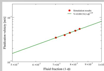
Fig. 3: The fluidization velocity vs. fluid fraction plotted in a log-log plot.
