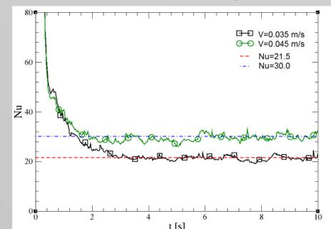
Fig. 6: Average Nusselt number of particles in a fluidized bed vs. time
