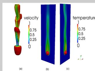
Fig. 4: Flow vortical structures (left) and temperature contours at Re=350.
