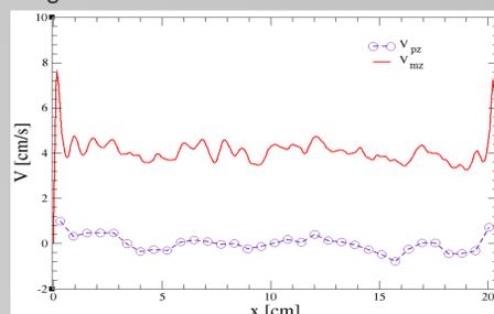
Fig. 2: time and z-direction averaged particle velocity and mixture velocity
