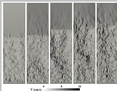
Fig. 1: Fluidization of 1204 spheres at five different velocities.
