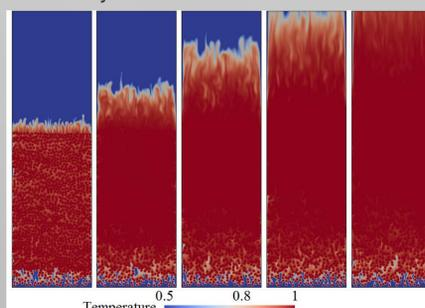
Fig. 5: Snapshots of temperature contours in a fluidized bed when V=4 cm/s. From left to right: t = 1s, 3s, 5s, 7s, and 10s
