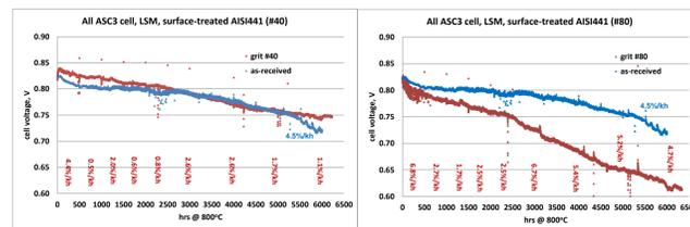
Cell with #40 grit-blasted showed stable/low degradation
