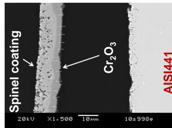
Cr-oxide scale de-bonded after ageing 4000h at 800°C in air of the as-received AISI441 coated with (Mn,Co)-spinel.
