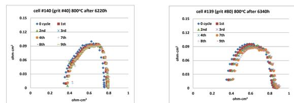
Minute increase in ohmic resistance suggests no substantial de-bonding of Cr-oxide scale
