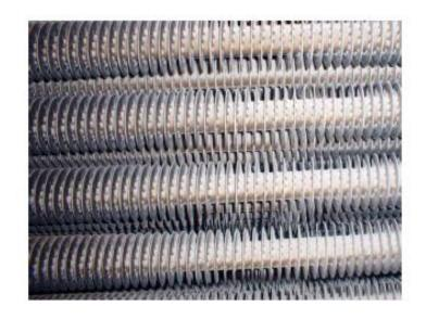
Carbon steel tubes in good condition after 2 years operation at Japanese plant
