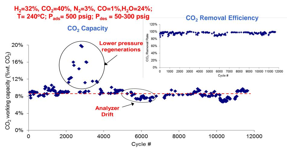
• Sorbent maintained its CO<sub>2</sub> capacity (8+%wt.) for 12,650 cycles
