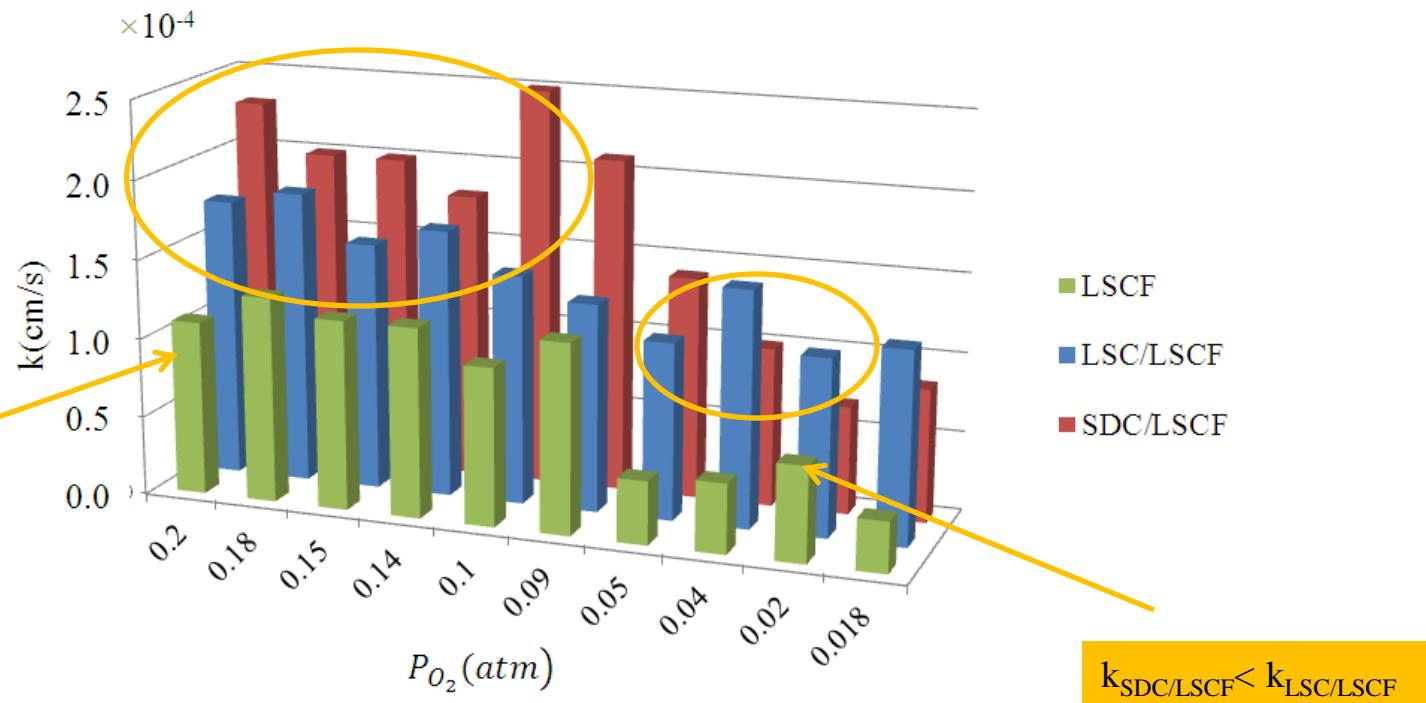
Surface exchange coefficients of single phase LSCF and infiltrated cathodes
