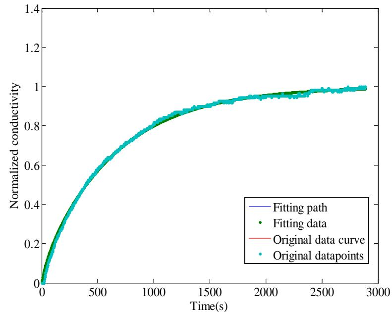
Normalized conductivity and fitting curve of spin coated LSC with oxygen partial pressure changing from 0.05atm to 0.04atm
