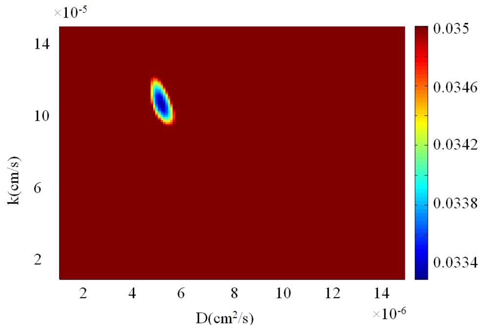
The estimation error for oxygen surface exchange coefficient was decreased by 80% within a 5% variation of minimum error band
