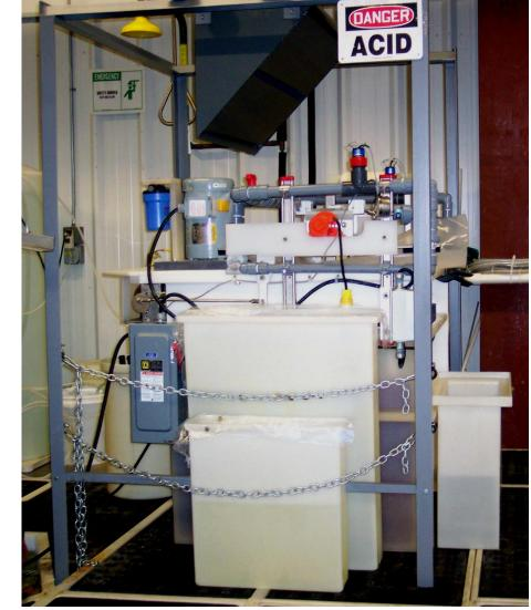
Modified FARADAYIC<sup>SM</sup> Electrodeposition Cell for coating patterned interconnect substrates ranging in size from 6.5 cm<sup>2</sup> to 625 cm<sup>2</sup>
