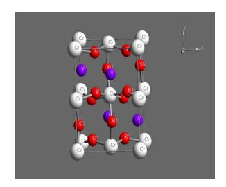
YCrO<sub>4</sub> and YCrO<sub>3</sub> structures used in our simulation. Both have rectangular structures. The blue balls stand for Y atoms, white balls for Cr atoms while red balls for O atoms.
