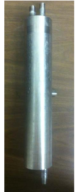
Module for lab testing (Ø2" x 15" long, 1m 2 )
