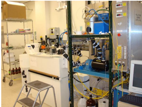
GE hollow fiber fabrication line
