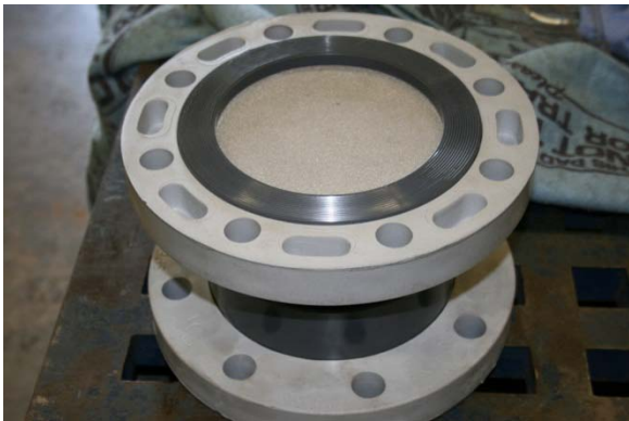
Distributor plate using a porous plate (Mott Corp.)
