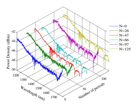
Experimental results showing the spectral evolution of a static LPG (with a period of 3mm) with increasing number of periods.
