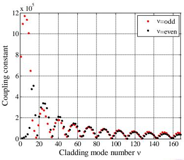
Analytical results showing the dependences of the grating period and the coupling constant on the corresponding cladding mode number.
