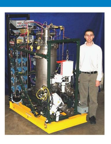
Modular, 250 kW<sub>e</sub> Fuel Processing System consisting of fuel/air/steam injector, ATR steam generator hex, and downstream sulfur clean-up
