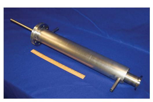
7.5 KWth CSR for up to 10 atm operation w. low sulfur diesel
