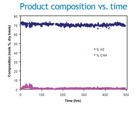
Operation w. distillate fuel containing 2-5 ppm<sub>w</sub> Sulfur
