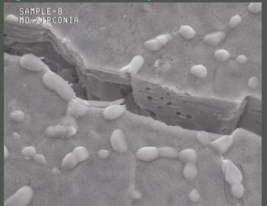
Exposed to Mo oxides, YSZ cracked
