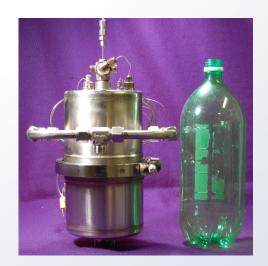
Convert JP-8\*/Diesel\* into sulfur free (< I ppm<sub>v</sub>) reformate
