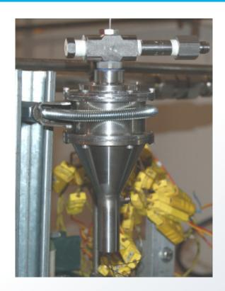
~30 cc reactor + fuel/air injector + igniter
