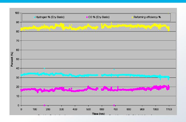
JP-8 w. low S (Average ~15 ppm $_{\rm w}$  S); Higher HC's < 20 ppm. Operated with I kW $_{\rm e}$  SOFC stack – Stable Operation w/o coking for I I00 hours
