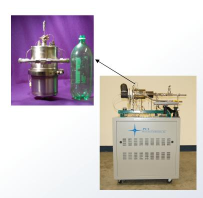
5 – 10 kW<sub>th</sub> reformer integrated w. fuel/air/steam injector, igniter, steam generating HX, sulfur trap. Cabinet w. balance of plant components (fuel, water tanks, pumps, contols, power supply, etc.)
