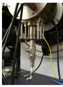
**SOFC Test** Fixture for **XRD**
