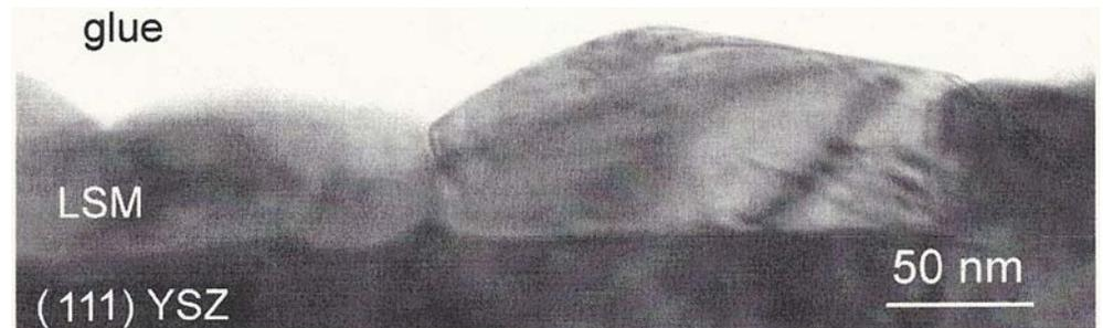
TEM image of annealed film and substrate.
