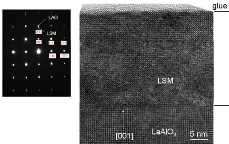
LSM on LAO [001]. Left: electron diffraction patterns. Right: HREM micrograph.
