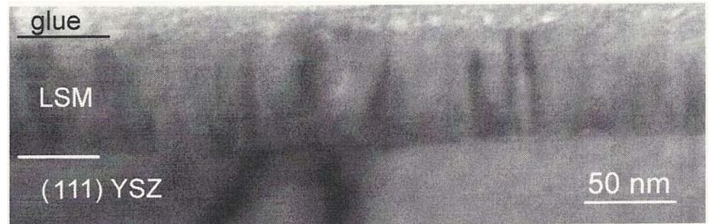
TEM image of as deposited film and substrate.
