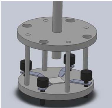
New setup allows measurement of surface exchange coefficient over a wide range of temperature and  $pO_2$
