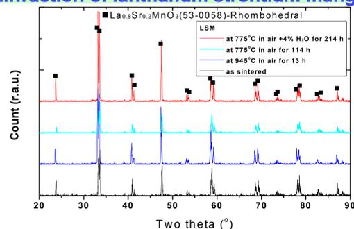
**Figure 2.** X-ray diffraction patterns of LSM pellets given different annealing conditions.
