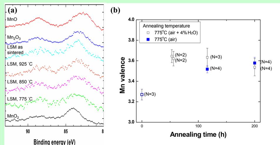
**Figure 3.** (a) Mn 3s XPS spectra (energy axis referenced to C 1s peak) of reference manganese oxide powders ( $\text{MnO}_2$ ,  $\text{Mn}_2\text{O}_3$  and  $\text{MnO}$ ) and LSM pellets annealed for 200 h in air at the indicated temperatures. The splitting of the doublet was used as a measure of the Mn valence in the LSM specimens as a function of (b) time and atmosphere.
