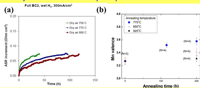
**Figure 1.** Effect of annealing temperature and time on (a) ASR of button cells and (b) Mn valence in LSM specimen.
