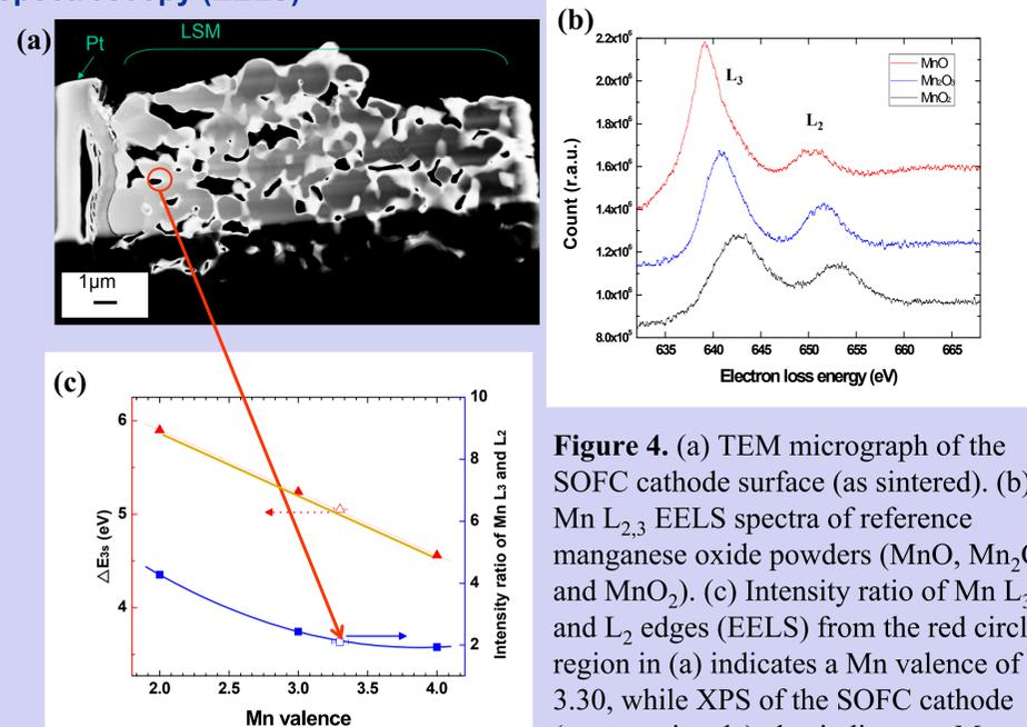
**Figure 4.** (a) TEM micrograph of the SOFC cathode surface (as sintered). (b) Mn L<sub>2,3</sub> EELS spectra of reference manganese oxide powders ( $\text{MnO}$ ,  $\text{Mn}_2\text{O}_3$  and  $\text{MnO}_2$ ). (c) Intensity ratio of Mn L<sub>3</sub> and L<sub>2</sub> edges (EELS) from the red circled region in (a) indicates a Mn valence of 3.30, while XPS of the SOFC cathode (orange triangle) also indicates a Mn valence of 3.30 from the splitting of the Mn 3s peak.
