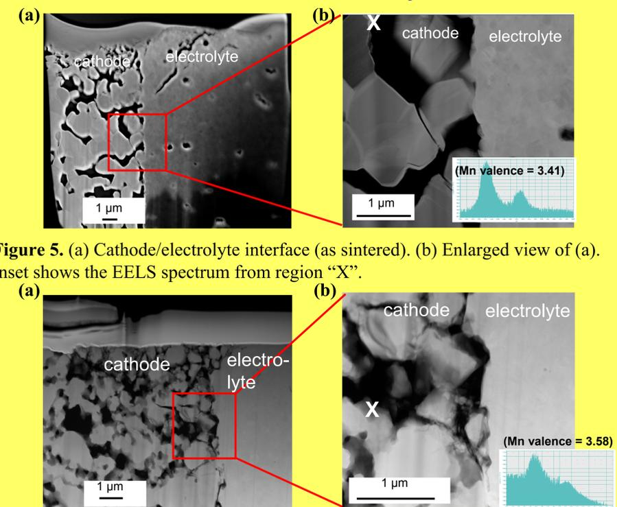
**Figure 5.** (a) Cathode/electrolyte interface (as sintered). (b) Enlarged view of (a). Inset shows the EELS spectrum from region "X".
