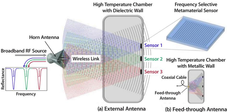
*Novel wireless sensors using radio frequency identification will allow measurement of temperature and pressure in harsh high-temperature environments.*
