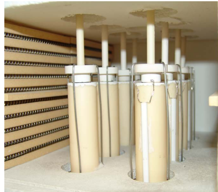
Eight button cells installed per box furnace, with individual gas flow controls
