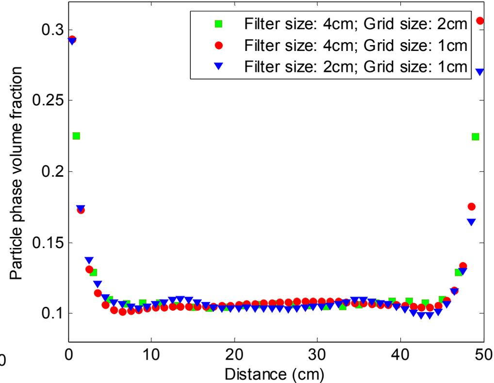
*Filtered model with closures corresponding to filter sizes of 2 and 4 cm yield nearly the same time-averaged results as long as grid size is less than equal to 0.5 (filter size)*
