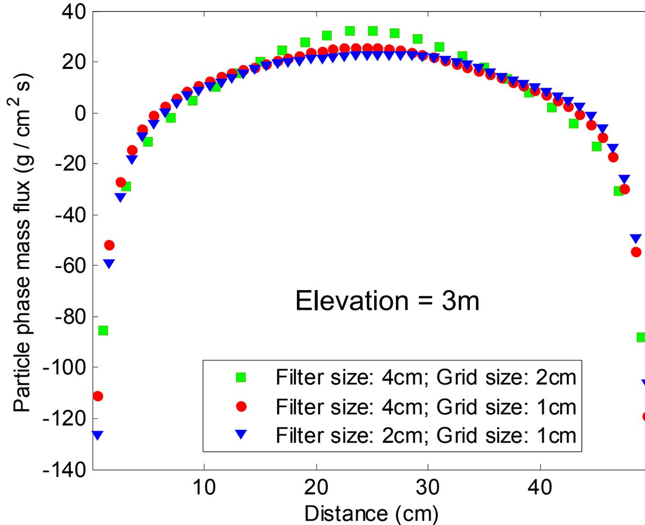
*Filtered model with closures corresponding to filter sizes of 2 and 4 cm*
