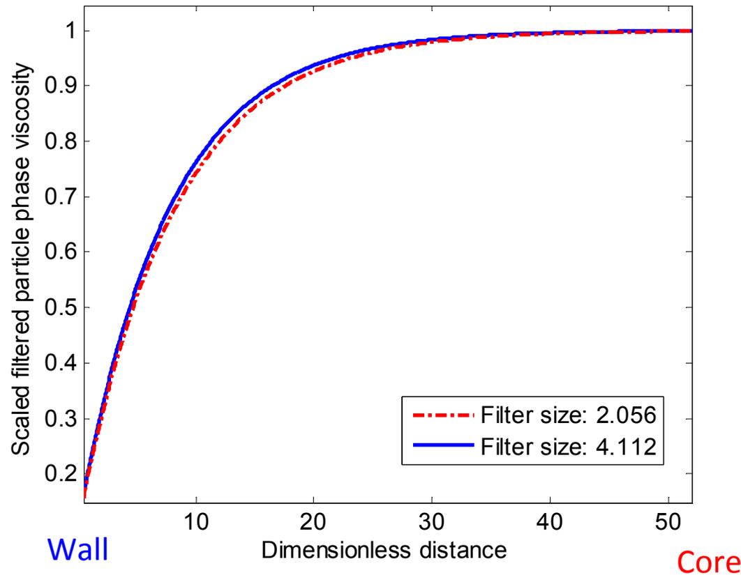
$$\overline{\mu_{s,filtered, scaled}} = \frac{\overline{\mu_{s,filtered, with wall correction}(\phi_s, r)}}{\overline{\mu_s^*(\phi_s)}}$$
