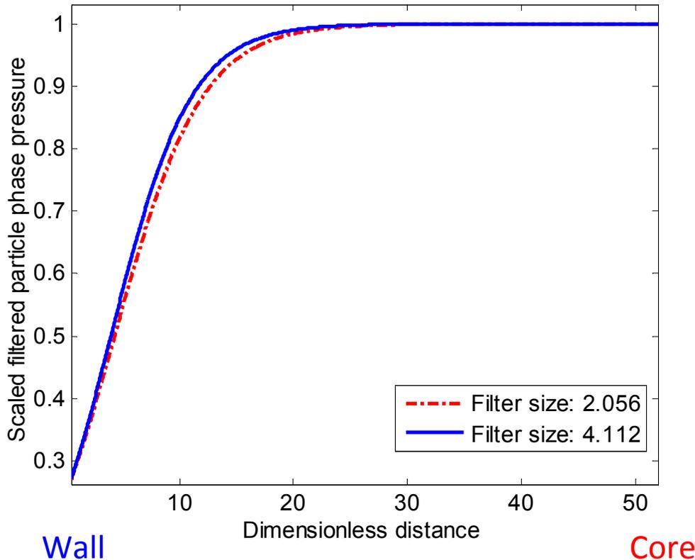
$$\overline{P_{s,filtered, scaled}} = \frac{\overline{P_{s,filtered, with wall correction}(\phi_s, r)}}{\overline{P_s^*(\phi_s)}}$$
