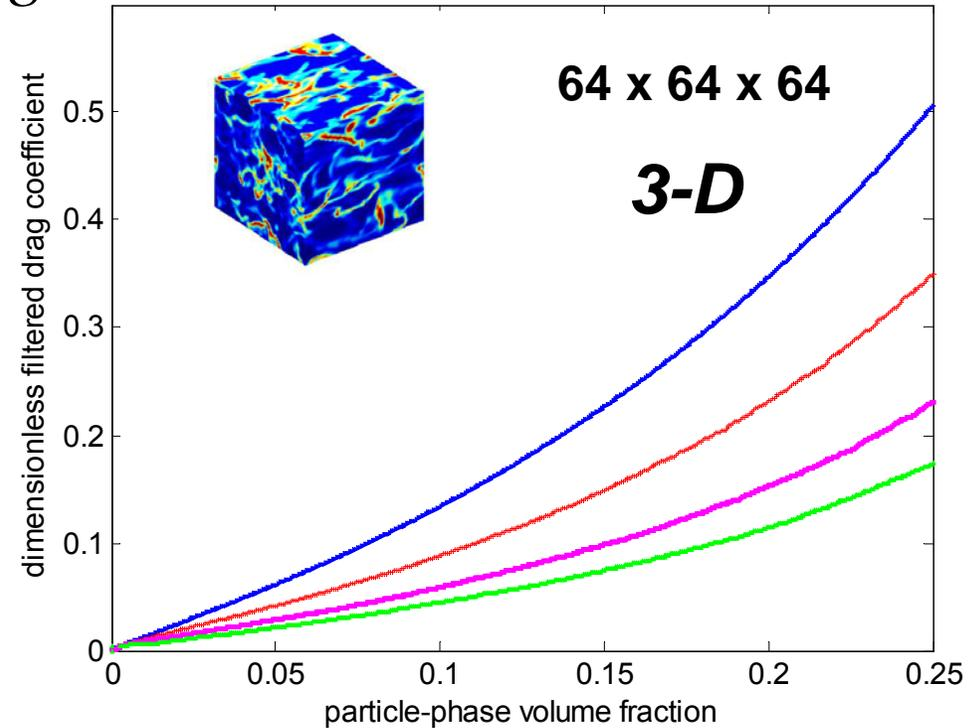
Example: 75  $\mu\text{m}$ ; 1500  $\text{kg}/\text{m}^3$ ; domain size = 8 cm
