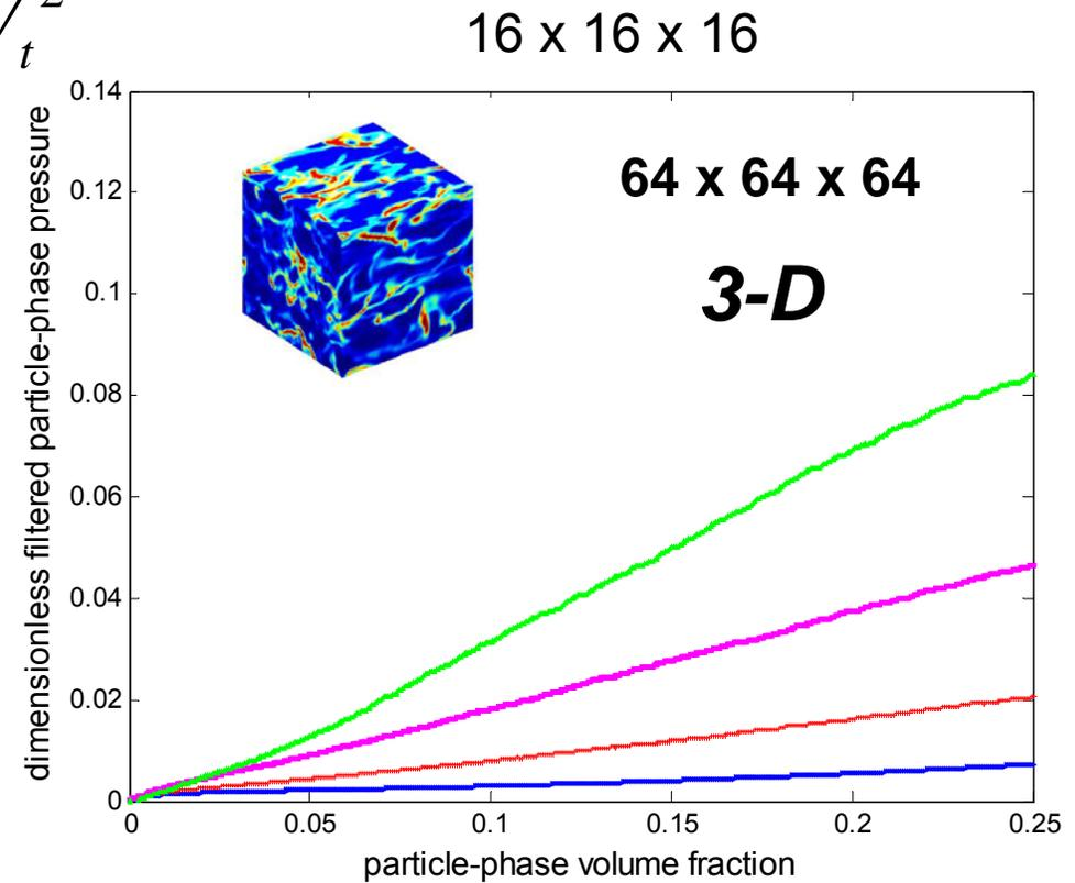
Example: 75  $\mu\text{m}$ ; 1500  $\text{kg}/\text{m}^3$ ; domain size = 8 cm
