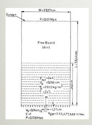
Bubbling Test Cases from *Multiphase* Flow and Fluidization, Gidaspow, p. 156.
