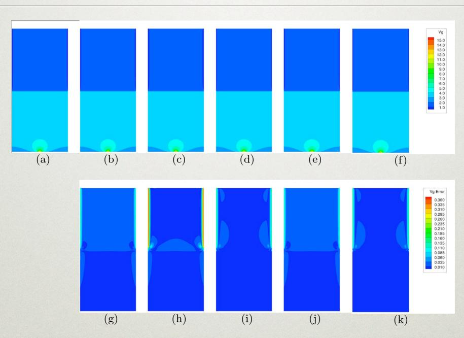
(a) FOM, (b) ROM, no acceleration, (c) ROM, matrix freezing, (d) ROM, database splitting, (e) ROM, initial time step adjustment, (f) ROM, database splitting and initial time step adjustment; and the gas velocity difference between (g) FOM and ROM, no acceleration, (h) FOM and ROM, matrix freezing, (i) FOM and ROM, database splitting, (j) FOM and ROM, initial time step adjustment, and (k) FOM and ROM, database splitting and initial time step adjustment (all values at t = 1.0 s).
