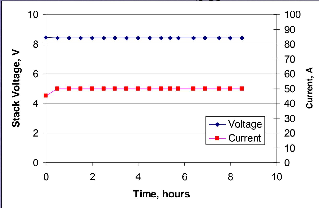
Steady state operation at 50 amps for eight hours using S-8 reformate and stoichiometric oxygen feed to the stack. At 50 amps, the single-pass fuel utilization was 35% and the oxygen utilization was 95%.
