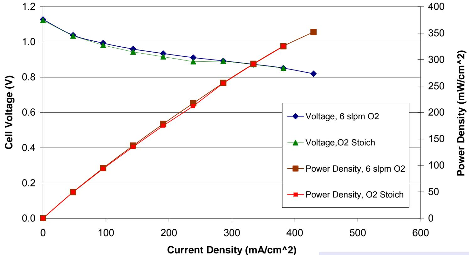
Comparison of IV plots shows that stoichiometric oxygen control has negligible effect on operating voltage.
