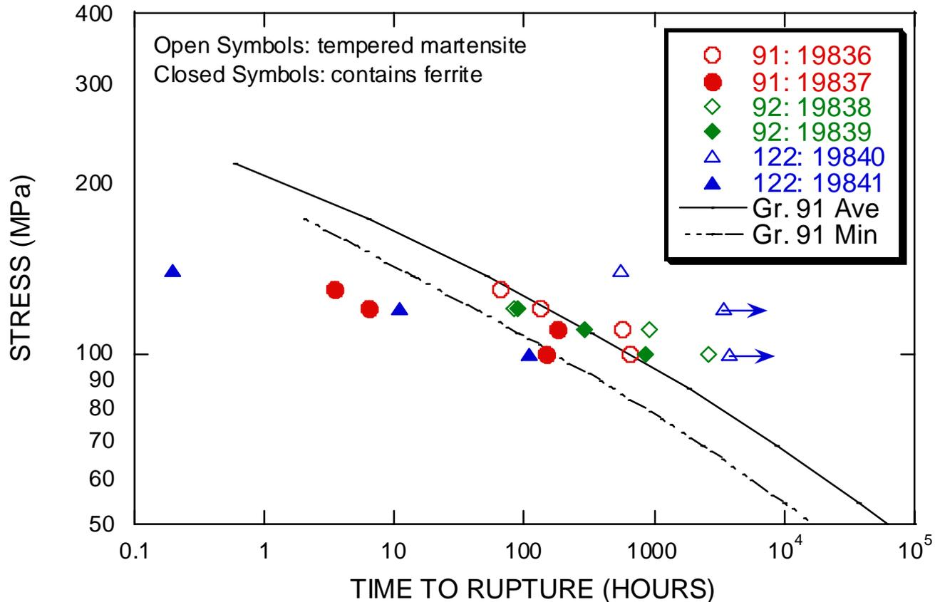
/// Alloy compositions should be controlled to avoid ferrite
