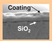
Investigation of interconnect coating/substrate degradation mechanisms
