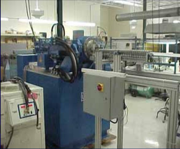
Anode Tube Extrusion
