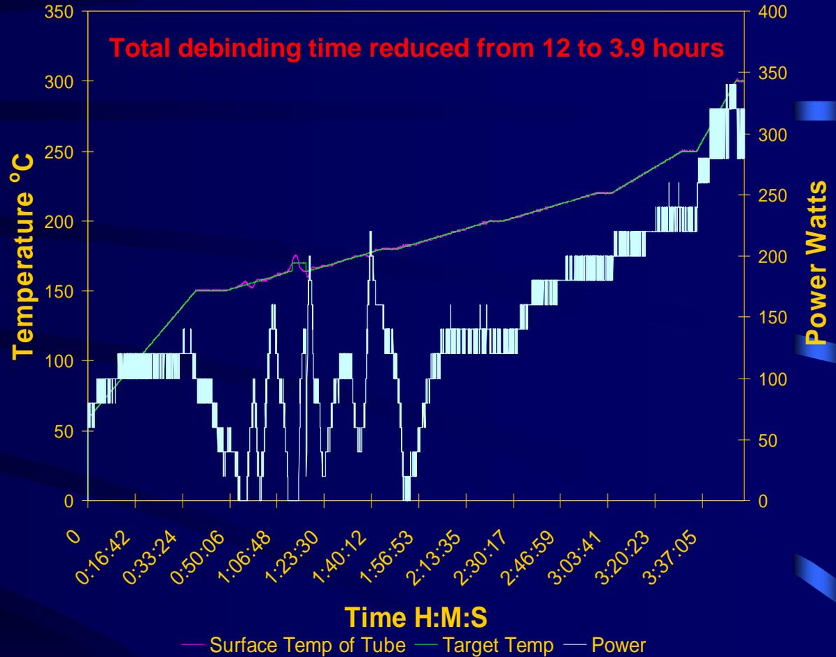
Light from optical pyrometer shines directly upon the part that is being debinded to allow constant temperature feedback and therefore adjustment of microwave energy giving optimum debinding time and conditions
